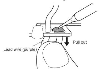
1. Unsolder the solder on purple lead wire from back side of the module and pull it out.
