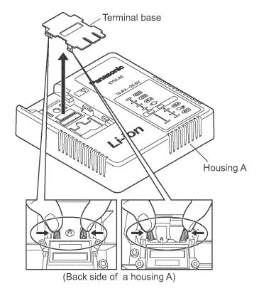
1. Remove the terminal base from the housing A.
