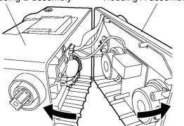
7. Use a pair of nippers to cut off the cable tie that holds the lead wires together.
