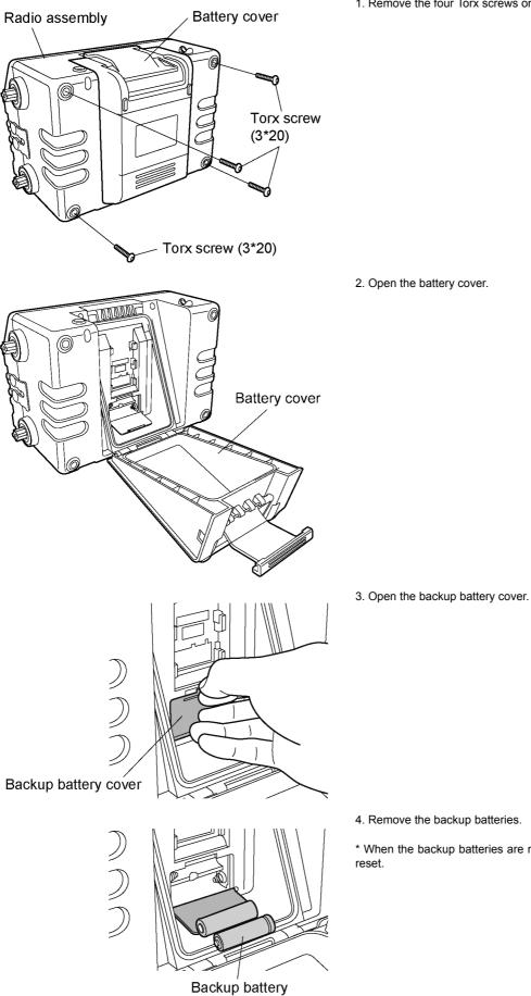
1. Remove the four Torx screws on the back of the radio assembly.
