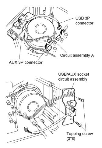
1. Disconnect the USB/AUX socket circuit assembly 3P connector and AUX 3P connector from circuit assembly A.
