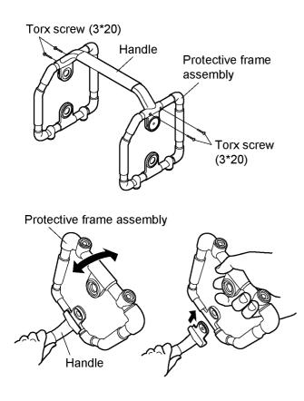
1. Remove the four Torx screws that connect the handle and the protective frame assembly.
