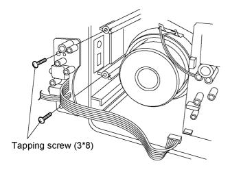
1. Disconnect the DC/EP socket circuit assembly 5P connector from circuit assembly A.
