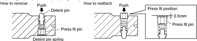
\* When replacing the detent pin, replace the entire set (detent pin, press-fit pin and detent spring). Note that Panasonic cannot guarantee that the replacement will fully recover the product performance. We recommend the replacement of the anvil block.
