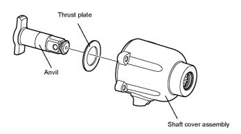
Remove the anvil from the shaft cover assembly and then remove thrust plate.
