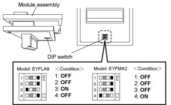
Check the settings of the DIP switches on the bottom Of the module assembly's control switch.
