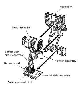
Remove the interior components from the housing A.
