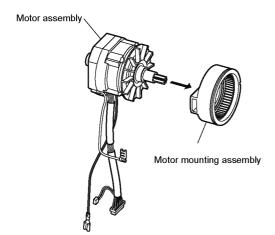
Remove the motor mounting assembly from the motor assembly.
